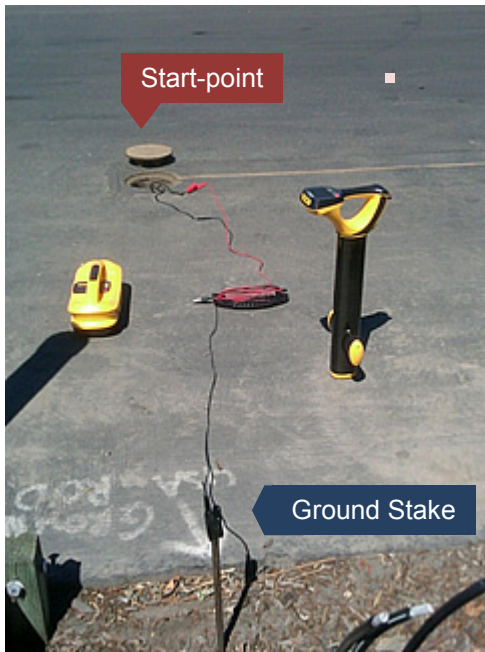
Figure 3. Instrument Hook up for Underground Facility
