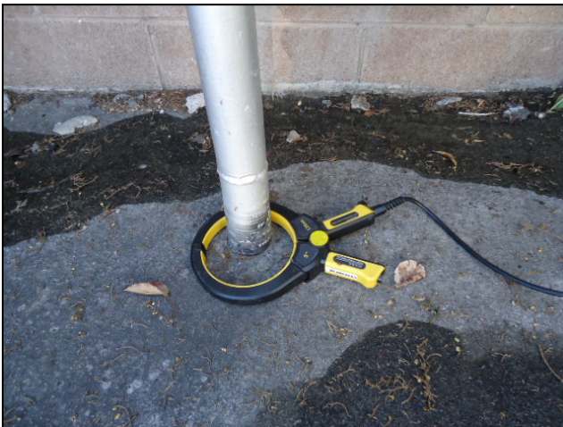
Figure 10. Inductive Clamp (Conductive Pipe)
