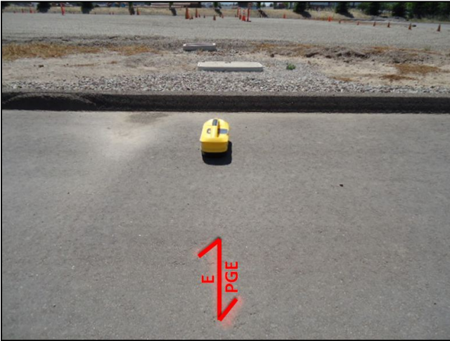
Figure 13. Inductive (Over the Top of a Facility)
