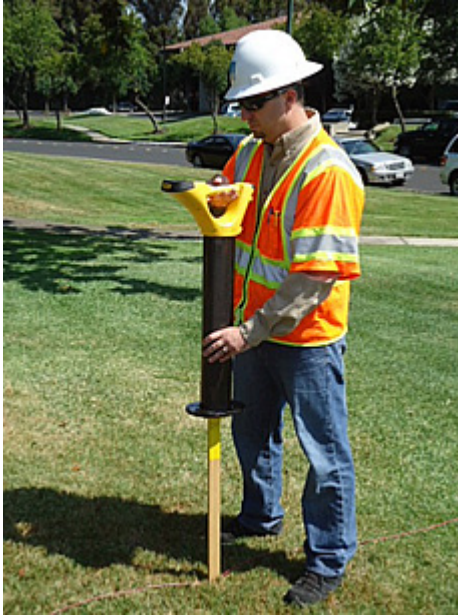
Figure 7. Determine Depth Using an Aboveground Facility
